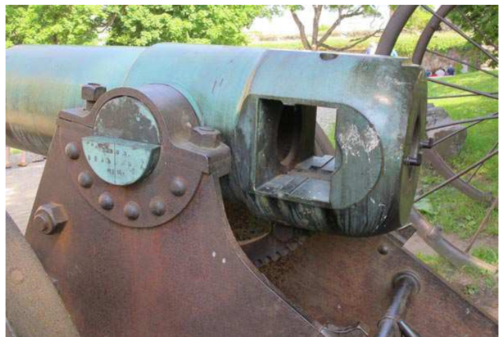
Curious breach on a cannon at the Finnish fort at Suomenlinna. Obviously a piece had to be inserted horizontally before the gun was fired.
