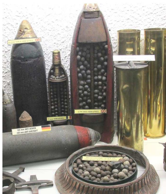
Showing Shrapnel inside shells.
