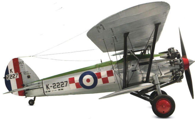
Bristol Bulldog 1929 (UK) Top speed: 178 mph The RAF's main day/night fighter between the wars. Cheap, good speed, twin guns.
